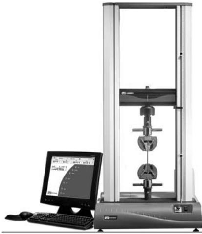
Fig. 3, Instron type 3366 tensile testing machine
