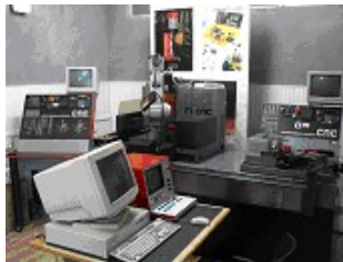
Fig.3. The flexible manufacturing EMCO CNC system
