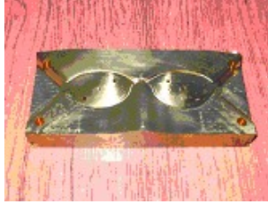
Fig.5. Active elements of an injection mould die for eyeglasses produced in the Computer Aided Manufacturing Laboratory
