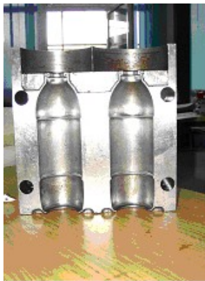
Fig.6. Active elements of an extruded mould produced in the Computer Aided Manufacturing Laboratory
